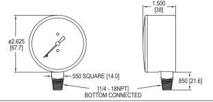
Our Series LPG4 2.5" Low Pressure Gage offers top of the line performance and accuracy for pressure and vacuum applications up to and including 160 in w.c. The LPG4 is constructed from a single beryllium-copper diaphragm affixed to a precisionmachined brass plate. This innovative design, together with a high-precision, milledteeth brass movement and nickel-silver pinion and bearing surface, provide the user with a top of the line low pressure instrument.
